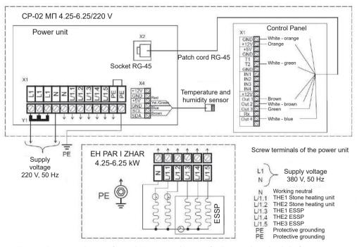
Fig. 6.2.2 Connection diagram of EH and CP 4.25 - 6.25 kW/220 V for the control panel with the four-wire sensor
