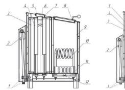
**Fig. 3** Design of heater 4,25; 6,25 kW
