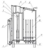
**Fig. 4.1** Design of heater 10,0; 12.0; 16,0 kW
