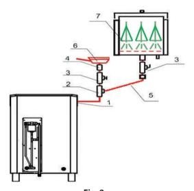
**Fig. 8**Diagram of herbal steamer and besom steamer connection.
