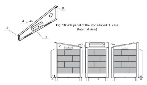
**Fig. 11.1** Layouts of the installation of decorative stone facing tiles for EH 4.25; 6.25 kW
