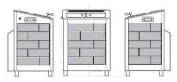
Fig. 11.1 Layouts of the installation of decorative stone facing tiles for EH 10-16 kW
