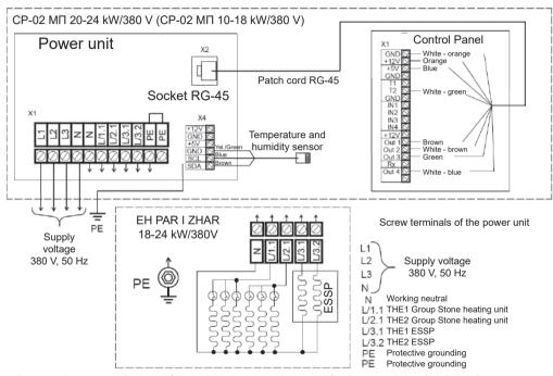
$\textbf{Fig. 6.8.1} \ Connection \ diagram \ of \ EH \ and \ CP \ 18.0 - 24.0 \ kW/380 \ V \ for \ the \ control \ panel \ with \ the \ three-wire \ sensor$
