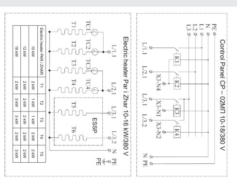
Fig. 6.5 Connection diagram for EH and CP 10,0-16,0 kW/380 V
