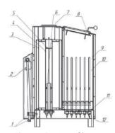
**Fig. 4.2** Design of heater 18,0; 20,0; 22,0; 24,0 kW
